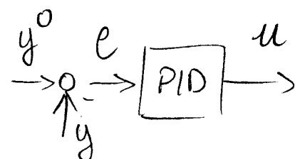
$$u(t) = \underbrace{K_p \cdot e(t)}_{\text{parte proporzionale}} + \underbrace{K_I \cdot \int_0^t e(\tau) d\tau}_{\text{parte integrale}} + \underbrace{K_D e(t)}_{\text{parte derivativa}}$$
