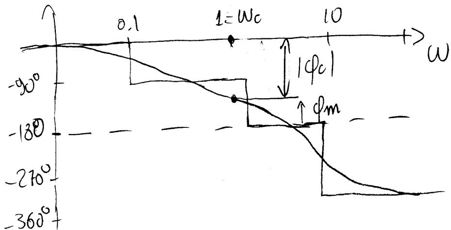
$$\begin{aligned}\varphi_c &= -\arctan(10 \cdot 1) - \arctan(0.5 \cdot 1) - 2\arctan(0.1 \cdot 1) = \\ &= -84^\circ - 26^\circ - 11^\circ = -121^\circ\end{aligned}$$
