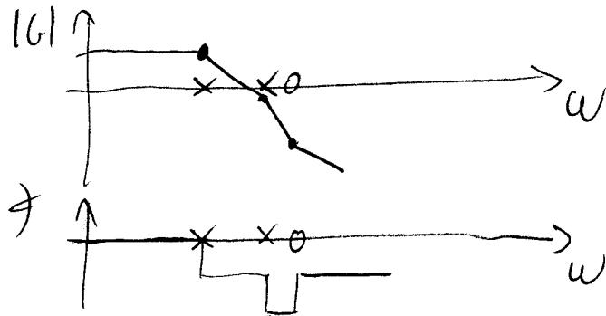
$$\bullet \text{Pase non minimo} \quad |G(j\omega)|_{\text{asint.}} \leq \frac{90^\circ}{20^{\text{dB}/\text{dec}}} \frac{d|G(j\omega)|/\text{dB}}{d\omega}$$
