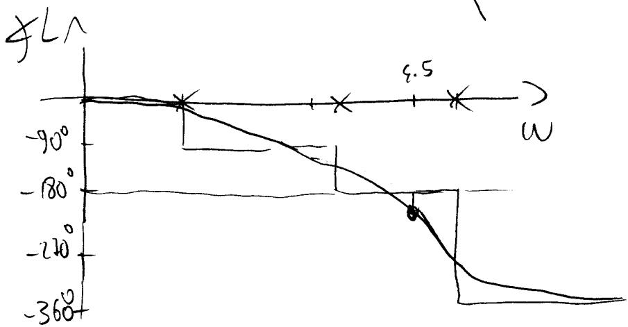
$$\begin{aligned}\varphi_c &= -\arctan(4.5 \cdot 10) - \arctan(4.5 \cdot 0.5) - \arctan(4.5 \cdot 0.1) = \\ &= -89^\circ - 66^\circ - 48^\circ = -203^\circ\end{aligned}$$
