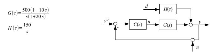
**5.1** Design a PI or PID controller with a bandwidth of 0.01 rad/s and at least 50° phase margin.
