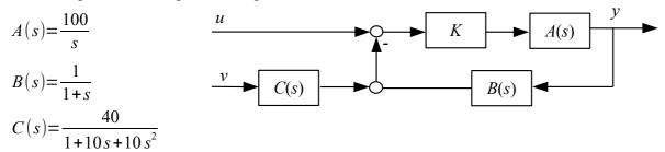
**4.1** Compute the transfer functions between the inputs u and v and the output y.
