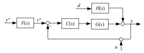
The feed-back controller C(s) must be designed to meet the specifications regarding disturbance rejection (both from d and from n). The pre-filter F(s) must then be designed so that
