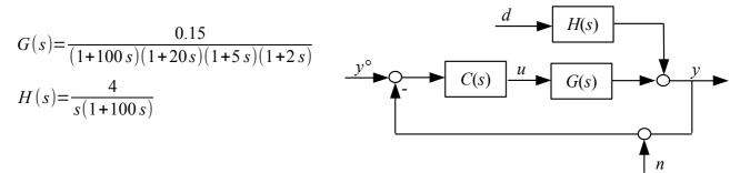
**3.1** Compute the steady-state errors corresponding to unit step changes of the set point  $y^{\circ}$  and of the disturbance d.
